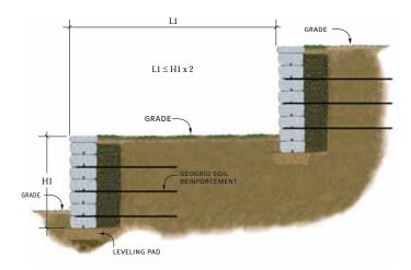
For walls where L1  $\geq$  H1 x 2, then the walls typically are analyzed separately. Walls built on slopes  $\geq$  3:1 or on soft soils need to be analyzed for "global stability". Consult a qualified engineer.
