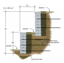
For walls where  $L1 \le H1 \times 2$ , then the walls are to be considered as a composite and the entire wall height (H) needs to be considered in the design.
